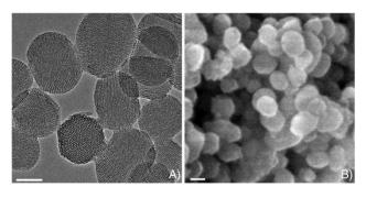
Figure 5. Mesoporous silica nanoparticles (MSNPs) used routinely in our laboratory. (A) and (B) represent unmodified MSNPs imaged by transmission and scanning electron microscopy, respectively. (Scalebar = 0.05 µm for A, and 0.1 µm for B). MSNPs exhibited homogenous size with slightly non-spherical shape and nanometre-sized pores with hexagonal symmetry. (Reproduced with permission from [93]).
