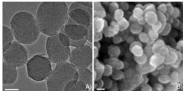
**Figure 5.** Mesoporous silica nanoparticles (MSNPs) used routinely in our laboratory. (A) and (B) represent unmodified MSNPs imaged by transmission and scanning electron microscopy, respectively. (Scalebar = 0.05 µm for A, and 0.1 µm for B). MSNPs exhibited homogenous size with slightly non-spherical shape and nanometre-sized pores with hexagonal symmetry. (Reproduced with permission from [93]).
