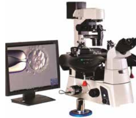
Figure 2: Full ART micromanipulator and laser system, featuring an inverted microscope fitted with a micro-manipulation stage, micro-manipulation tools, and infra-red laser. The stage, laser, and laser software shown here are manufactured by Research Instruments Ltd (UK). Image courtesy of Research Instruments Ltd (reproduced with permission)
