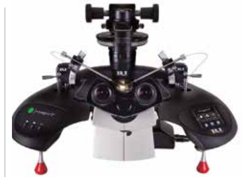
Figure 3: Precise embryo micromanipulation tools fitted onto an Integra micromanipulation stage (Research Instruments Ltd UK). Image courtesy of Research Instruments Ltd (reproduced with permission)
